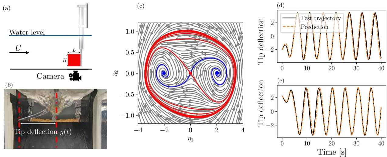
**Fig. 5 | Reduced model of the inverted flag experiment.** **a** Experimental setup of the inverted flag and snapshot of the experiment **(b)**, courtesy of Giovanni Berti. The geometric parameters are  $H = 150$  mm,  $L = 150$  mm,  $U = 1$  m/s. **c** Phase portrait of the gSSM-reduced dynamics of the inverted flag obtained from the  $[5/5](\boldsymbol{\eta})$  approximation. The unstable fixed points are marked with colored dots. Blue
