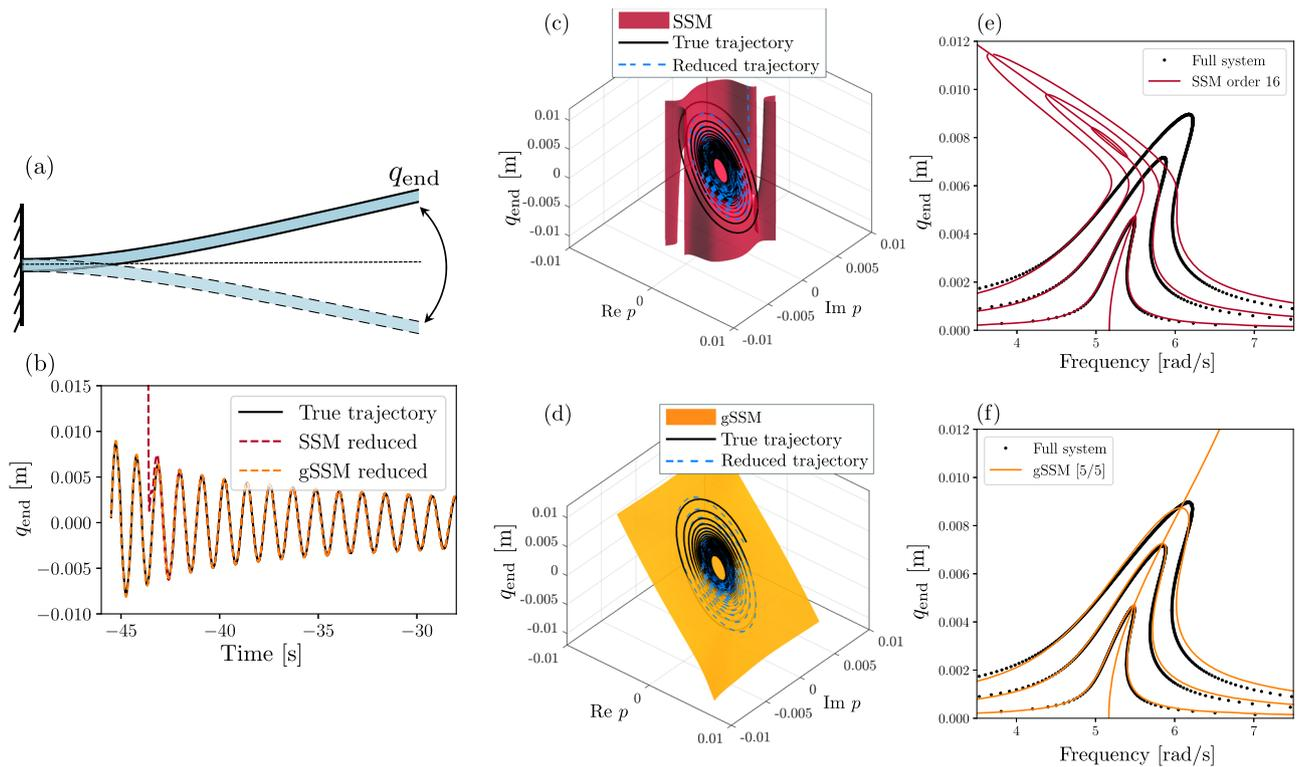
**Fig. 2 | Model reduction of a von Kármán beam.** **a** von Kármán beam with clamped-free boundary conditions. **b** Trajectory of the unforced system (black) with its order-16 SSM approximation (red) and gSSM-approximation (orange) with a [5/5] and [5/4] Padé approximant. **c, d** Representation of the end point displacement  $q_{end}$
