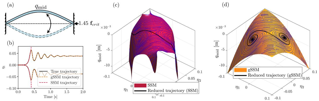
**Fig. 3 | Reduced model of the buckled beam.** **a** Sketch of the beam in the buckled configuration, with no external forcing. **b** Trajectories in the unstable manifold of the unstable fixed point (black). Their order-18 SSM-reduced (red) and order [6/6] gSSM-reduced (orange) approximations are also shown. **c, d** The SSM and gSSM in
