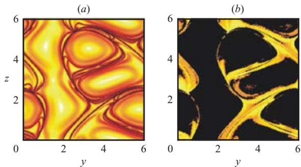
FIGURE 10. Visualization of the intersection of vortices with the  $x = 2\pi$  plane in the ABC flow. (a) Finite-time Lyapunov exponents over the time interval  $[0, 10]$ , with darker colours indicating higher values. (b) Time spent in the domain where  $M_Z$  is indefinite; if the time is at least 90% of the entire simulation interval  $[0, 10]$ , the trajectory is coloured black.
