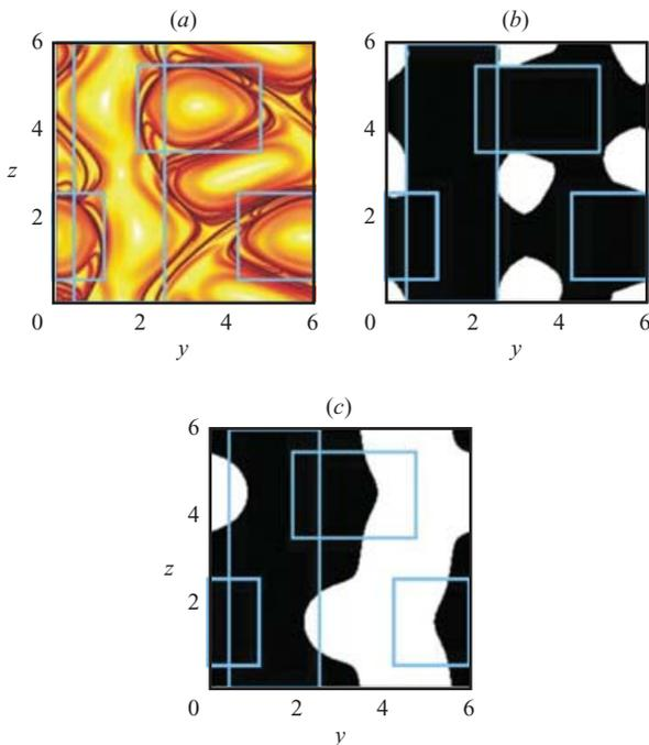
FIGURE 11. The rough location of vortices (marked by rectangles) as inferred from the Lyapunov exponent plot (a), then superimposed on the elliptic region shown in (b), and on the  $\lambda_2 < 0$  region shown in (c).
