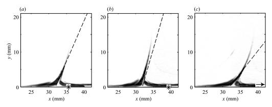
FIGURE 7. Separation spike in 5.97 mm r.m.s. quasi-periodic flow compared with the numerical prediction for: (a) an intermediate angle (t = 52.3 s); (b) a large angle (t = 73.0 s); (c) a small angle (t = 79.0 s). (\*) or ( $\rightarrow$ ) indicates the location of the instantaneous zero-skin-friction point.
