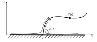
FIGURE 1. A time-dependent unstable manifold  $\mathcal{M}(t)$  originating from the fixed separation point  $p = (\gamma, 0)$  making angle  $\alpha(t)$  with a no-slip boundary.
