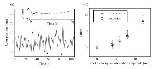
FIGURE 6. (a) 5.97 mm r.m.s. amplitude quasi-periodic rotor location (main plot line) and convergence of the fixed separation location,  $\gamma$  (inset); (b) the fixed separation location,  $\gamma$ , as a function of the r.m.s. amplitude of oscillation for quasi-periodic forcing.
