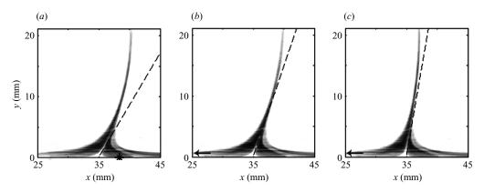
FIGURE 5. Separating material spike in periodic flow (24 mm peak-to-peak oscillation amplitude) compared with the numerical prediction (dashed line) for: (a) minimum separation angle (t = 2.0 s); (b) intermediate separation angle (t = 3.7 s); (c) maximum angle (t = 5.0 s). (\*) or ( $\leftarrow$ ) indicates the location of the instantaneous zero skin-friction point.
