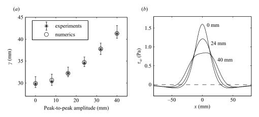
FIGURE 4. (a) Comparison of the experimental and numerical separation location,  $\gamma$ , for periodic forcing. (b) Mean skin-friction profiles for 0 mm, 24 mm and 40 mm peak-to-peak amplitude oscillations. Where the profiles cross the dashed line identifies points of zero mean skin-friction.
