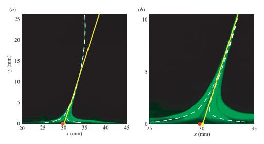
FIGURE 3. (a) The separating material spike in steady flow. (b) Enlargement of the material spike in (a). Superimposed on the images are numerical streamlines (white dashed lines), the experimental separation location (red circle), and the predicted separation profile (yellow line) originating from the predicted separation location (yellow circle).
