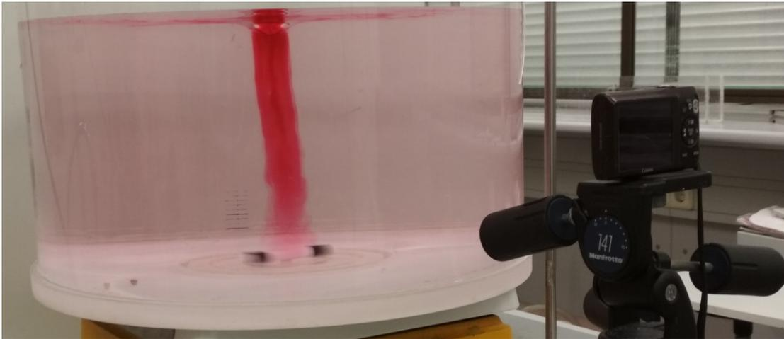
FIGURE 1. A coherent material vortex visualized experimentally by dye. Image: courtesy of M. Vincze and T. Tél. See Tél et al. (2018) for details on the experiment.
