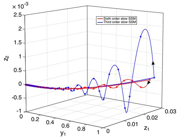
**Fig. 9** Poincaré map for trajectories launched on different approximation to the slow SSM. *Dots* indicate intersections of the trajectories with the  $y_2 = 0$  hyperplane. *Arcs* connecting adjacent intersections are for illustration only, to give a sense of the trajectory evolution
