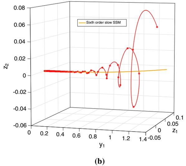
**Fig. 15 a** Fast convergence of a generic trajectory to the slow SSM and then subsequently to the equilibrium point along the SSM. Initial conditions for the trajectory were chosen off the SSM with the coordinates  $y_1(0) = 1.2, y_2(0) = 0, z_1(y_1(0), y_2(0)) + \Delta z_1 = -0.042 + 0.1, z_2(y_1(0), y_2(0)) + \Delta z_2 = -0.0045 + 0.1$ . The vertical axis in the figure represents
