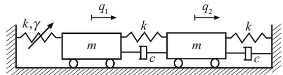
**Fig. 6** The two-degree-of-freedom mechanical model considered by Shaw and Pierre [39]
