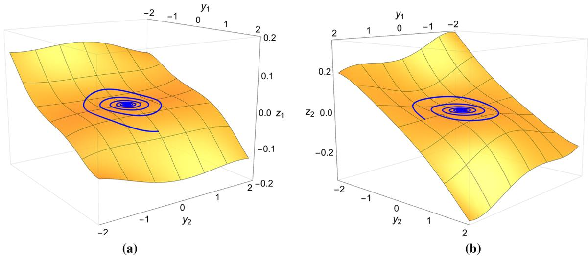
**Fig. 8** Two views of the slow SSM for the nonlinear oscillator system (38)–(39). In the plots (8a–8b),  $z_1$  and  $z_2$  are shown as a function of  $y$ , respectively. The *blue curve* is a trajectory starting on the SSM from the initial conditions  $(y_1(0) = 1.2, y_2(0) =$
