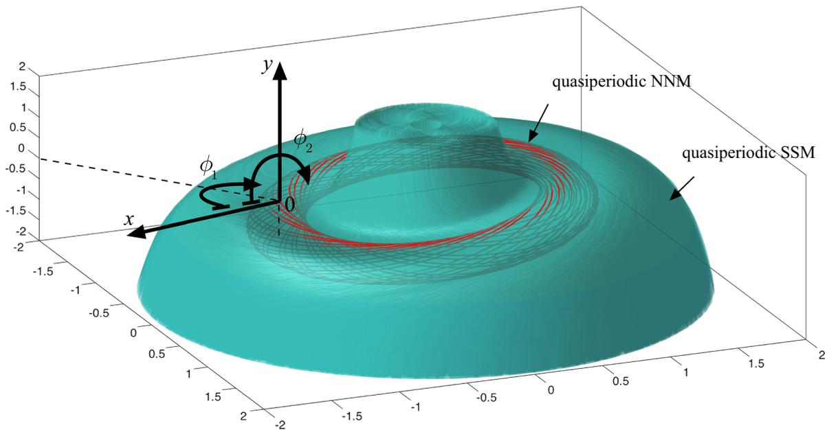
**Fig. 11** A projection of system (53) from the extended phase space of  $(x, y, \phi_1, \phi_2)$ , where  $\phi_1 = (\phi_{10} + \Omega_1 t) \bmod 2\pi$  and  $\phi_2 = (\phi_{20} + \Omega_2 t) \bmod 2\pi/\sqrt{2}$ . The green surface is the unique analytic, quasiperiodic SSM guaranteed by Theorem 4, emanating from the unique quasiperiodic NNM (red) guaranteed
